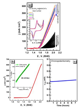
(a) CV measurements for UiO-66-NH2-Ni@MWCNTs (colored traces) with the inset showing the Ni(II/III) redox couple, and the Ni@MWCNTs control (black trace), (b) LSV scan showing the OER activity of the composite with the Tafel plot and linear fit in the inset, and (c) controlled current electrolysis for 7 h. Measurements were conducted in aerated 1 M KOH solution, with a scan rate of 100 mV s<sup>-1</sup> for the CVs and 10 mV  $\rm s^{-1}$  for the LSV.
