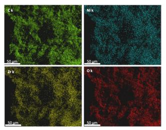
**Fig. 3** EDX maps for UiO-66-NH<sub>2</sub>-Ni@MWCNTs showing the homogenous distribution of the elements (labeled images) throughout the sample.
