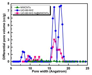
Fig. 7 Pore size distribution (PSD) histograms for the UiO-66-NH<sub>2</sub>, MWCNTs, and UiO-66-NH2-Ni@MWCNTs.
