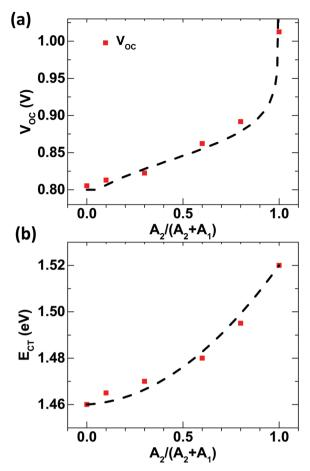
Fig. 2 Alloy composition vs. (a) changes in  $V_{\rm OC}$  using the double-diode model (the dotted line represents the fitting of experimental  $V_{\rm OC}$  values with eqn (2)) and (b) changes in the  $E_{\rm CT}$  value of the BHJ alloy composition determined from sensitive EQE studies (the dotted line represents the fitting of experimental  $E_{\rm CT}$  values with eqn (3).
