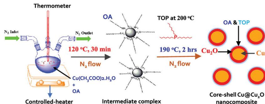
Fig. 9 Schematic of the synthesis process of Cu@Cu<sub>2</sub>O core-shell nanoparticles using copper acetate hydrate, oleylamine (OA), and trioctylphosphine (TOP). Reproduced with permission from ref. 112, Copyright 2020 American Chemical Society.
