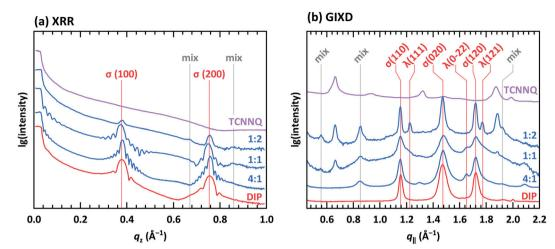
Fig. 8 (a) X-ray reflectivity (XRR) and (b) grazing incidence X-ray diffraction (GIXD) measurements for single component and co-deposited films of DIP and TCNNQ. The peaks donated as  $\sigma(\lambda)$  are related to phases containing upright standing (lying) DIP molecules. Peaks marked as "mix" are attributed to the formed mixed crystal. Corresponding respective reciprocal space maps are shown in ESI† (see Fig. S1)
