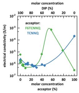
**Fig. 10** Electrical conductivity determined at room temperature for single component and co-deposited D:A films of DIP, TCNNQ and F6TCNNQ as function of the molar concentration measured. The solid lines are given to quide the eyes.
