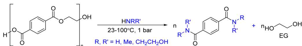
Fig. 34 Typical reaction conditions and products for PET aminolysis.
