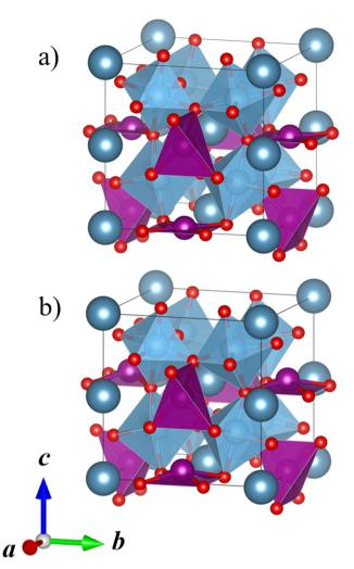
**Fig. 5** (a) Calculated lowest-energy structure of CaMnTi<sub>2</sub>O<sub>6</sub> ( $P4_2/nmc$ ,  $E_{\rm rel} = 9$  kJ mol<sup>-1</sup> per formula unit). (b) Experimental ferroelectric CaMnTi<sub>2</sub>O<sub>6</sub> structure with the square-planar Mn cations displaced ( $P4_2mc$ ,  $E_{\rm rel} = 0$  kJ mol<sup>-1</sup> per formula unit). <sup>21</sup> Ca ions colored in dark grey-blue, Mn ions in purple, Ti ions and their coordination polyhedra in blue, and oxygen anions in red.
