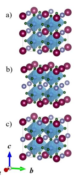
Fig. 2 A-site ordered double perovskites with (a) columnar, (b) planar, and (c) rock salt ordering. The two cation species on the A-site are shown in dark red and purple, the B-site cations and their coordination polyhedra in blue, and the X-site anions in green. The unit cell in each system is drawn in black.
