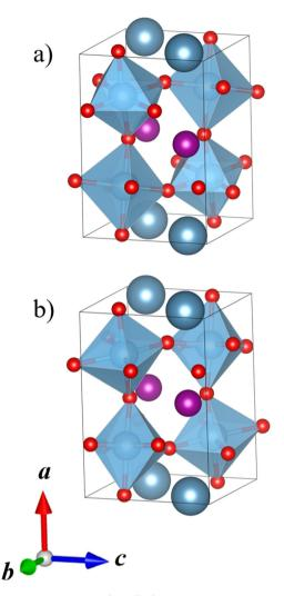
Fig. 3 Two tilt systems of CaMnTi<sub>2</sub>O<sub>6</sub> with planar A-site ordering (space group P2/c): (a)  $a^-b^-b^-$  and (b)  $a^-a^-a^-$ . Ca ions colored in dark grey-blue, Mn ions in purple, Ti ions and their coordination polyhedra in blue, and oxygen anions in red.
