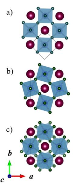
**Fig. 1** Perovskites with different Glazer tilt systems along the c direction: (a) ideal, untilted, (b)  $a^0a^0c^+$ , and (c)  $a^0a^0c^-$ . The A-site cations are in dark red, the B-site cations and their coordination polyhedra in blue, and the X-site anions in green. The unit cell in each system is drawn in black. All crystal structure illustrations in the manuscript have been prepared with the VESTA program.<sup>8</sup>
