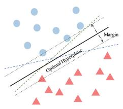
Fig. 10 Scheme of the SVM classification with a hyperplane. Blue dots and red triangles represent the training instances with two labels. The black line represents the optimal hyperplane, which maximizes the margin between the blue and red instances. The red and blue dash lines are hyperlines that can separate the two groups apart, though the corresponding margin is less than the optimal one.
