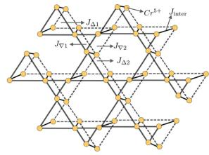
**Fig. 31** The crystal structure showing only the  $Cr^{5+}$  ions in  $Ca_{10}Cr_7O_{28}$ . Five different interaction matrix elements as illustrated in eqn (116) are depicted. Reprinted from A. Kshetrimayum, C. Balz, B. Lake and J. Eisert, Tensor network investigation of the double layer Kagome compound  $Ca_{10}Cr_7O_{28}$ , Ann. Phys., 2020, **421**, 168292, Copyright (2022), with permission from Elsevier.
