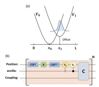
Fig. 38 (a) Graphical description of the Marcus model; and (b) quantum circuit representation for the time evolution of the wave packet. The blocks represent the evolution operators shown in the form of quantum gates. CQFT,  $V_i$ , K and C correspond to centred quantum Fourier transform (used to switch from position to momentum space), ith potential, and Kinetic and coupling terms, respectively. Figure adapted from ref. 610.
