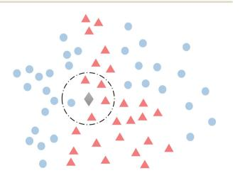
Fig. 5 A simple example of the kNN algorithm approach. The blue dots and red triangles represent the training instances with two labels, and the grey diamond is a new test instance. In this example k is set as 5, and the 5 nearest instances are included in the black circle. As there are 4 red triangles and only 1 blue dot, the class of the test instance is classified as a red triangle
