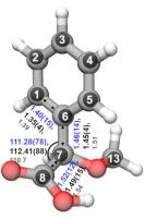
Fig. 7 Comparison of the calculated  $r_e$  (outer semi-transparent structure) and experimentally determined  $r_s$  substitution (black inner spheres) structures of cis-in-perp. The bond lengths and angles for the  $r_s$  structure are shown in black, for  $r_0$  in blue, and for  $r_e$  in gray.
