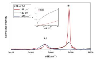
Fig. 2 Cryo-SEVI spectra of NiO<sub>2</sub> at three photon energies illustrating the differing signal attenuation for features A1 and B1 as eKE decreases. The intensity of each scan has been normalized to feature A1. Photon energies employed are 25 991 (blue),  $25\,001$  (black), and  $24\,728$  cm<sup>-1</sup> (red). Insert: photodetachment cross-section as a function of kinetic energy for s- and p-wave detachment as outlined by the Wigner threshold law.6
