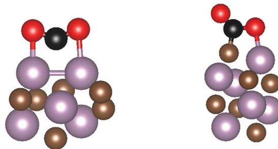
Fig. 3 Atomistic views of the  $\eta^3\text{-CO}_2\text{-}\mu^2\text{-C}_B\text{O}_M\text{O}_M$  (left) and  $\eta^2\text{-CO}_2\text{-}\mu^2\text{-C}_C\text{O}_M$  (right) adsorption modes seen on two different carbide nanoparticles. C, Mo and O atoms are shown as brown, magenta, and red spheres, respectively. The C atom in  $\text{CO}_2$  is shown as a black sphere.
