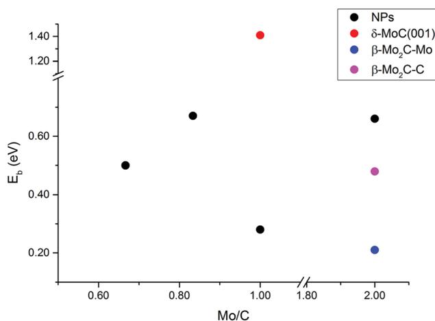
Fig. 9 Energy barrier ( $E_b$ ) for CO<sub>2</sub> dissociation on nanoparticles (NPs) at different Mo/C ratios. Data of  $\delta$ -MoC(001) and  $\beta$ -Mo<sub>2</sub>C(001) surfaces are included for comparison.  $\beta$ -Mo<sub>2</sub>C(001) Mo- and C-terminations are shown as  $\beta$ -Mo<sub>2</sub>C-Mo and  $\beta$ -Mo<sub>2</sub>C-C, respectively.
