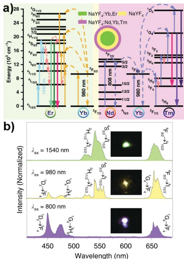
Fig. 2 (a) Proposed multiple excited state absorption and energy transfer mechanism in  $\text{Nd}^{3+}$ ,  $\text{Yb}^{3+}$ ,  $\text{Er}^{3+}$ , and  $\text{Tm}^{3+}$ -codoped UCNC.<sup>76</sup> (b) Upconversion emission spectra of UCNCs shown in (a) and the corresponding photo of UCNC films excited using  $\lambda_{\text{ex}} = 800$ , 980 and 1540 nm laser excitation.<sup>76</sup> Reprinted with permission from ref. 76. Copyright 2020, Nature Publishing Group.
