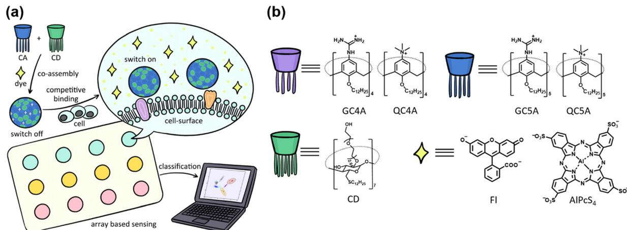
**Scheme 1** (a) Illustration of the construction of heteromultivalent macrocyclic coassemblies, the corresponding cell recognition by indicator displacement assay and cell discrimination by differential sensing. (b) Chemical structures of the employed CA, CD hosts and the reporter dyes.
