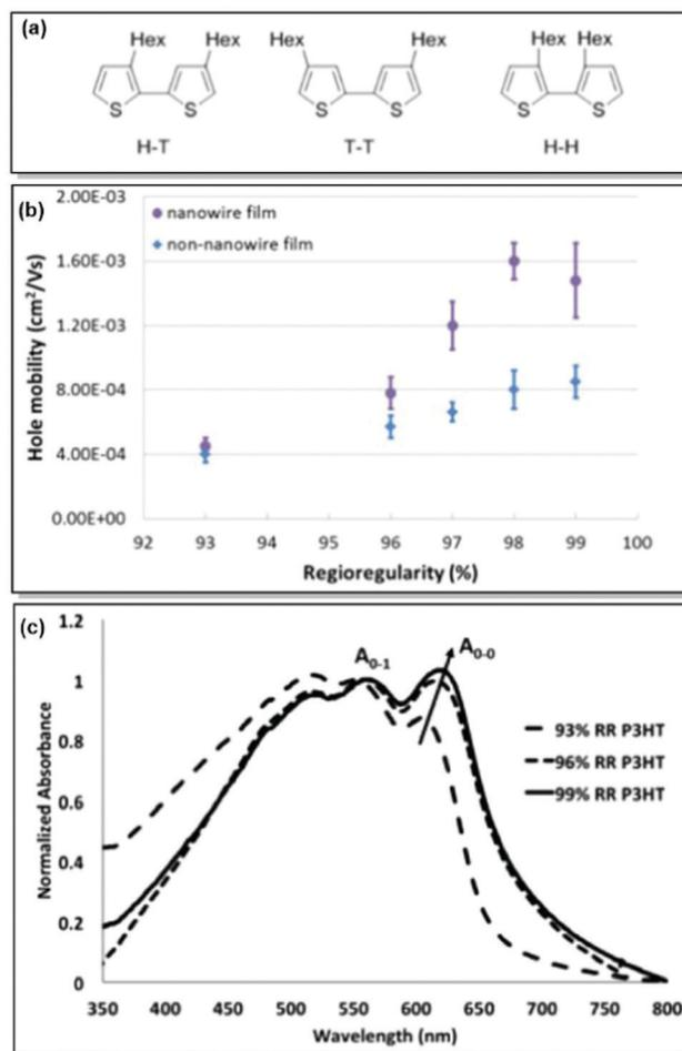
Fig. 2 (a) Possible coupling products of **P3HT** (H–T: head-to-tail, T–T: tail-to-tail, H–H: head-to-head). (b) Correlation between RR and hole mobility for **P3HT** nanowire and non-nanowire films. (c) UV-Vis absorption spectra for **P3HT** with various RR%. Reproduced with permission from American Chemical Society.<sup>67</sup>
