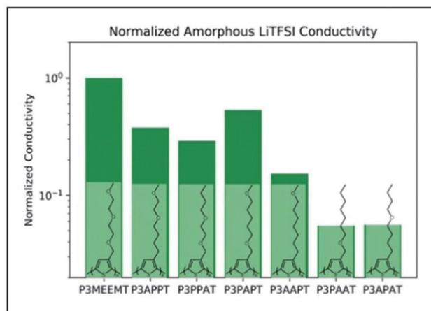
Fig. 7 Chemical structures of **P3MEEMT**, **P3APPT**, **P3PPAT**, **P3PAPT**, **P3AAPPT**, and **P3APAT** along with the calculated ionic conductivity values for amorphous polymer samples, normalized with the respective polymer dissociation energies, and further normalized against the **P3MEEMT** performance. Reproduced with permission from Royal Society of Chemistry.<sup>82</sup>
