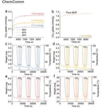
Fig. 3 CO<sub>2</sub> capture performance of (a) hybrid aerogels with different MOF loadings and (b) pure MOF, (c-f) weight changes for three consecutive cycles of CO<sub>2</sub> sorption-desorption of hybrid aerogels with 30%, 40%, 50% MOF and pure MOF, respectively.
