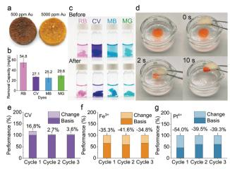
Fig. 4 Water purification performance. (a) Reduced Au<sup>3+</sup> into Au nanoparticle and metallic gold on top of the aerogel. (b and c) Dye removal performance. (d) Rapid removal of organic solvents from water. (e-g) Changes of adsorption performance after three regeneration cycles.
