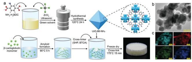
Fig. 1 Fabrication process of hybrid UiO-66-NH2 and amyloid fibrils aerogel. (a) Schematic of UiO-66-NH2 synthesis, and the preparation process of the hybrid aerogel. Morphological features of UiO-66-NH<sub>2</sub>. (b) TEM image of UiO-66-NH<sub>2</sub>. (c) Elemental maps of UiO-66-NH<sub>2</sub>.
