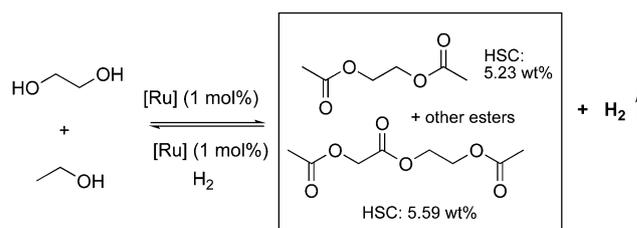
Fig. 27 Liquid organic hydrogen carrier system based on EG and ethanol.
