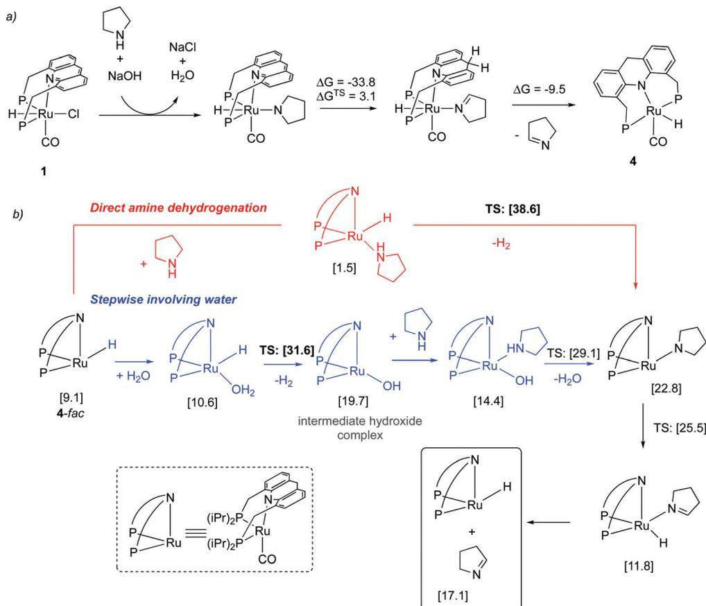
Fig. 20 (a) Initial dearomatization of complex **1** (b) amine dehydrogenation *via* direct (red) and stepwise pathway involving water (blue). Calculated free energies (in brackets) are in kcal mol<sup>-1</sup> with respect to **4-mer** + amine + water.
