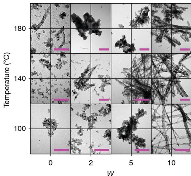
Fig. 18 TEM micrographs as a deep eutectic-solvothermal synthetic phase diagram for  $\text{CeO}_2$  nanoparticles post-calcination, where scale bars depict 100 nm, and  $w$  is the  $\text{H}_2\text{O}/[\text{DES}]$  molar hydration ratio. Reprinted with permission from Springer Nature.<sup>307</sup>
