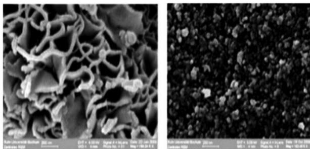
Fig. 3 NiO prepared in the IL 1-butyl-3-methylimidazolium bis(trifluoromethanesulfonyl)amide (left) and in aqueous solution (right). Reproduced with permission from RSC.<sup>43</sup>
