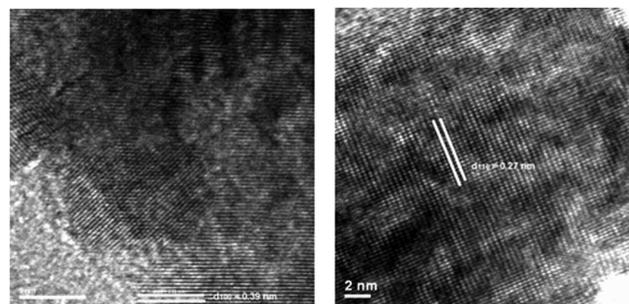
Fig. 11 HRTEM images of the as-prepared SrTiO<sub>3</sub> in [C<sub>3</sub>mimOH][Tf<sub>2</sub>N] with {100} expressed (left) and in [C<sub>4</sub>mim][Tf<sub>2</sub>N] with expression of {110} (right). Reprinted with permission from Wiley-VCH.<sup>156</sup>
