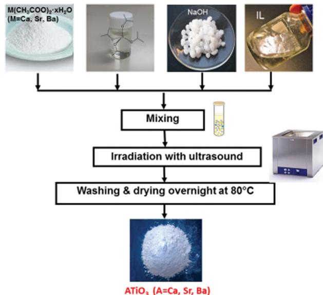
Fig. 10 Sonochemical ambient condition preparation of perovskite photocatalysts.
