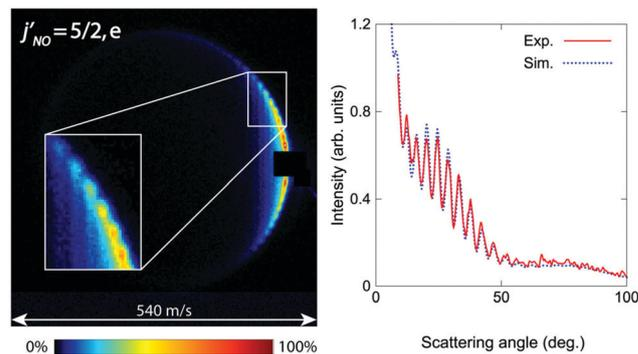
Fig. 3 Velocity map scattering image recorded following inelastic collisions between  $\text{NO}(X^2\Pi_{3/2}, j = 3/2)$  and Ne. Oscillatory patterns due to matter wave diffraction can be observed. As can be seen in the right hand side plot, excellent agreement was found between the experimental and simulated results. Adapted with permission from Plomp *et al.*, copyright American Institute of Physics, 2020.<sup>61</sup>
