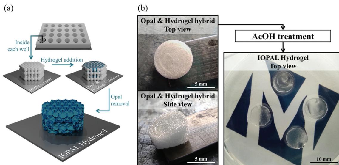
**Fig. 1** Formation of the IOPAL PEG–Hep hydrogel. (a) Simplified scheme of the formation of an IOPAL PEG–Hep hydrogel. (b) Photographs of the opal & hydrogel hybrid before the AcOH treatment, when they are white and opaque. After AcOH treatment, they result in transparent hydrogels, indicating the complete removal of the PMMA beads.
