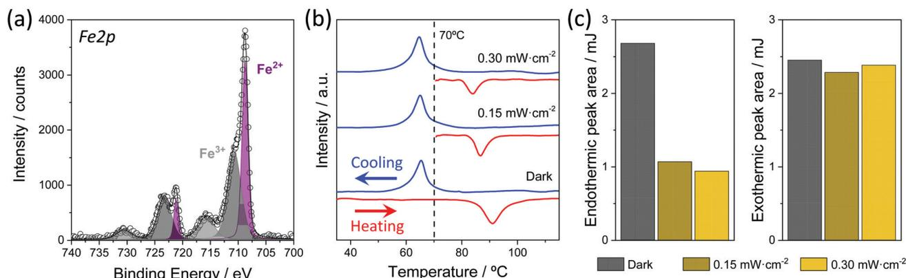
Fig. 4 (a) XPS spectra of the Fe region for NS@SCO NPs. (b) DSC curves of NS@SCO; the red line indicates the heating mode and the blue line represents the cooling mode. (c) Variation of the endothermic and exothermic areas in different conditions.
