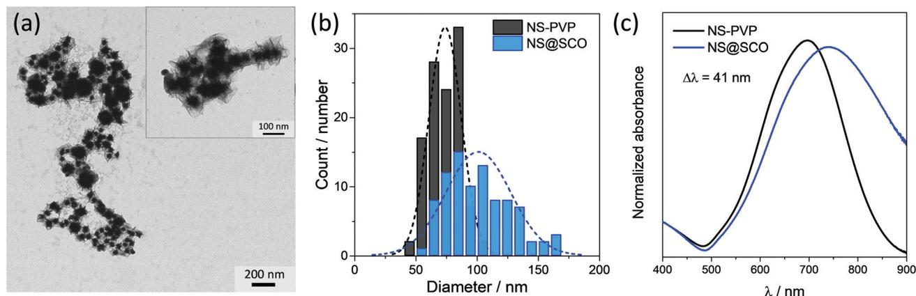
Fig. 2 (a) TEM images of the NS@SCO heterostructure and (b) histograms of the size distributions for the gold core (black) and the overall core@shell nanoparticle diameter (red). These sizes have been calculated from manual counting of more than 100 NPs. (c) UV-vis spectra of the NS@SCO and the NS NPs.
