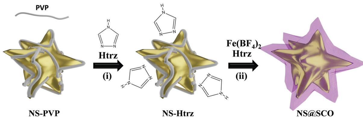
Fig. 1 Scheme of the synthetic protocol followed to obtain the NS@SCO core@shell nanoparticles. The synthesis consists of a previous Au surface modification followed by the sequential addition of the SCO precursors.
