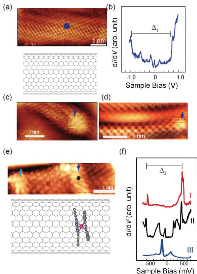
**Fig. 5** (a) STM image and (b) STS spectra of empty SWCNT. (c) and (d) STM images of TbPc<sub>2</sub>@SWCNT. (e) STM image showing empty (red) and filled (black) regions. (f) Comparative STS spectra measured at the red and black points in (e).
