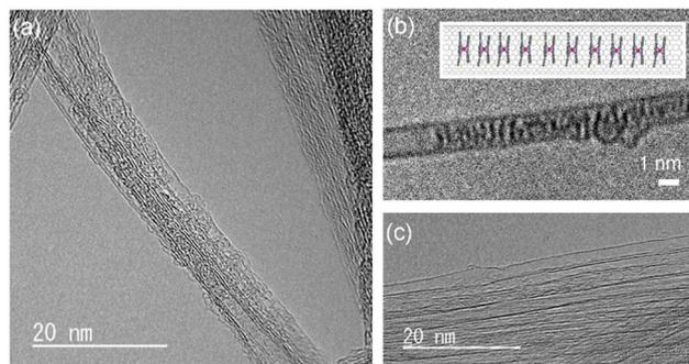
Fig. 2 Structural characterization of TbPc<sub>2</sub>@SWCNT. Conventional bright field and phase contrast TEM images of TbPc<sub>2</sub> encapsulated in SWCNTs. (a) TbPc<sub>2</sub> was confirmed to be inside SWCNTs. Tb was detected by using EDX (see Fig. S3, ESI<sup>†</sup>). (b) TbPc<sub>2</sub> were partially stacked one-dimensionally in SWCNTs. (c) Empty SWCNT.
