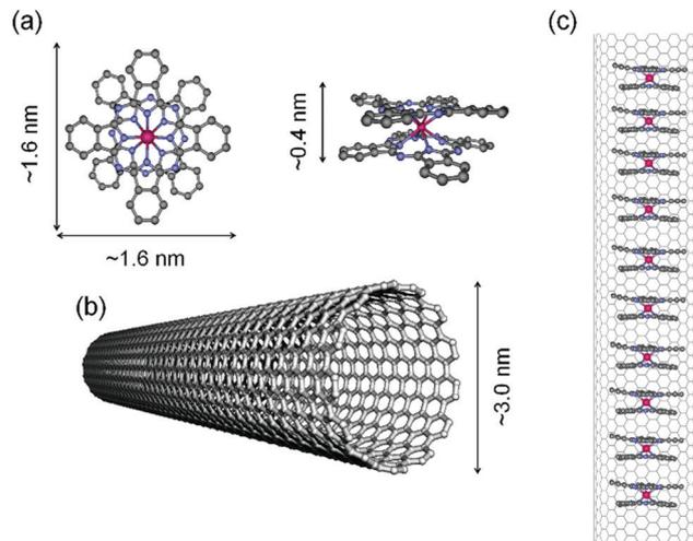
**Fig. 1** Chemical structure of  $\text{TbPc}_2$  SMM and schematic illustration of its encapsulation in SWCNTs. (a) Ball and stick structure of  $\text{TbPc}_2$ . Hydrogen atoms omitted for clarity: top (left) and side (right) view. Colouring scheme:  $\text{Tb}^{3+}$ , pink; N, cyan; C, grey. (b) Ball and stick structure of SWCNTs. (c) Schematic illustration of the  $\text{TbPc}_2$  SMM encapsulated in a SWCNTs (abbreviated as  $\text{TbPc}_2@mSWCNT$ ).
