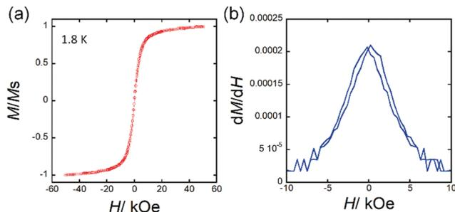
**Fig. 4** (a)  $M$ - $H$  curve and (b)  $dM/dH$  versus  $H$  plot for TbPc<sub>2</sub>@SWCNT at 1.8 K. The vertical axis,  $M/M_s$ , shows magnetization values normalized to the saturated magnetization value. The butterfly-type magnetic hysteresis seems to be closed in (a), but it is slightly open which was confirmed by using magnetic field differentiation of  $M$  in (b). The lines are guides for eyes.
