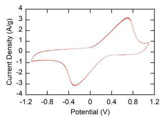
Fig. 2 Cyclic voltammetry of the P1-CNT/Ti electrode's final 10 cycles (from over 100 cycles) in the presence of 100 mM NaClO<sub>4</sub>. The potential range chosen was from  $-1.1\,\text{to}\,1.1\,\text{V}$  with a scan rate of 50 mV s  $^{-1}$ .
