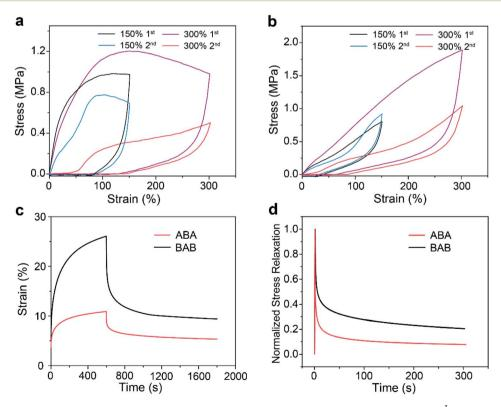
Fig. 4 Successive cyclic tensile curves of ABA (a) and BAB (b) at different strains (deformation rate: 100 mm min<sup>-1</sup>). (c) Creep-recovery response of the two triblock copolymers. (d) Stress relaxation curves of the two triblock copolymers.
