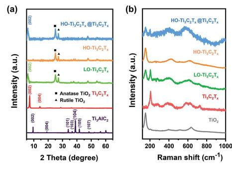
Fig. 2 (a) XRD patterns of  $Ti_3AlC_2$  powder and the dried films of  $Ti_3C_2T_x$ ,  $LO-Ti_3C_2T_x$ ,  $HO-Ti_3C_2T_x$ ,  $HO-Ti_3C_2T_x$ @ $Ti_3C_2T_x$ . (b) Raman patterns of  $Ti_3C_2T_x$ , LO- $Ti_3C_2T_x$ , HO- $Ti_3C_2T_x$ , HO- $Ti_3C_2T_x$ @ $Ti_3C_2T_x$  and  $TiO_2$  films.
