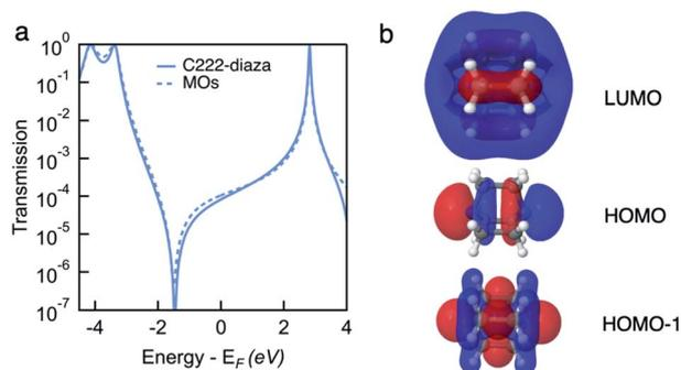
Fig. 4 (a) Transmission functions of C222-diaza, calculated as  $T(E) = |t_{\text{LUMO}} + t_{\text{HOMO}} + t_{\text{HOMO-1}}|^2$  (dashed line) overlaid with Landauer transmission in the wide-band limit (solid). (b) MOs of C222-diaza calculated using DFT with B3LYP functional. White, black and blue atoms represent H, C and N, respectively.
