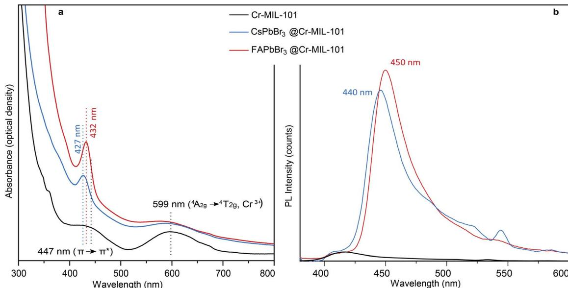
Fig. 4 (a) Absorbance and (b) photoluminescence spectra for nano-Cr-MIL-101, CsPbBr<sub>3</sub>@nano-Cr-MIL-101, and FAPbBr<sub>3</sub>@nano-Cr-MIL-101.
