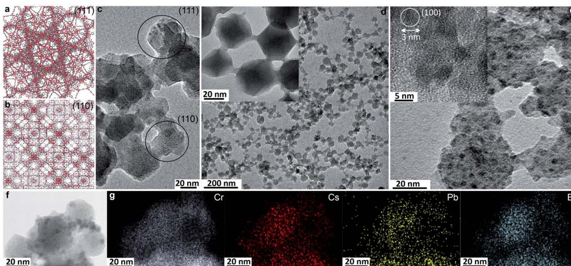
Fig. 2 (a) View of the (111) plane in Cr-MIL-101, (b) view of the (110) plane in Cr-MIL-101, (c) and (d) TEM images for nano-Cr-MIL-101 (approx. 25 nm NPs), (e) TEM images for CsPbBr<sub>3</sub>@nano-Cr-MIL-101 (approx. 25 nm NPs), (f) STEM image for CsPbBr<sub>3</sub>@nano-Cr-MIL-101. (g) STEM EDX mapping for CsPbBr<sub>3</sub>@nano-Cr-MIL-101.
