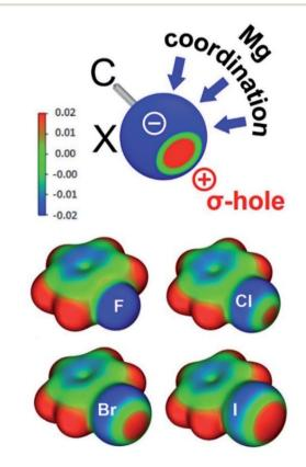
Fig. 2 (Top) Schematic representation of the  $\sigma$ -hole and possible coordination sites for Mg. (Bottom) Electrostatic maps of PhF, PhCl, PhBr and PhI at an isosurface of 0.003 a.u. of the total electron density.
