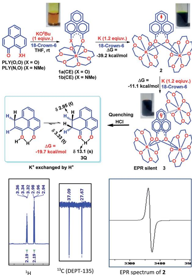
Scheme 1 Preparation of the PLY–K complexes (1a(CE) and 1b(CE),  $12\pi e^-$  species) and consecutive one electron reduction by K to generate mono-reduced  $13\pi e^-$  species (2) and doubly reduced  $14\pi e^-$  species (3), respectively; quenching the  $14\pi e^-$  species by replacing all  $K^+$  ions with  $H^+$  ions through HCl treatment; (insets: EPR spectrum of 2 and selected part of  $^1H$  and  $^{13}C$  (DEPT-135) NMR spectra of 3Q).
