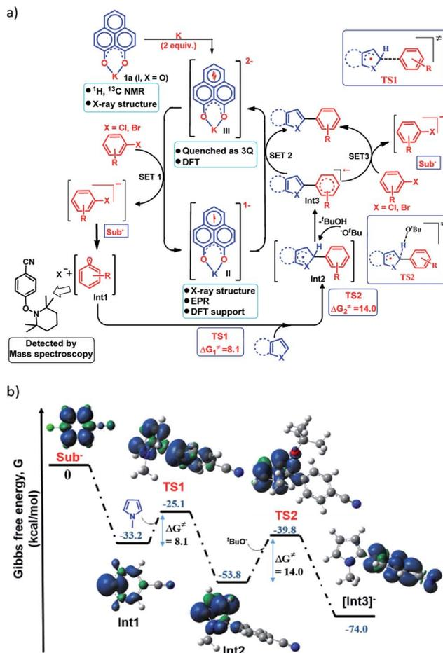
**Fig. 4** (a) Proposed mechanistic cycle for the C–H arylation reaction by aryl halide activation; (b) reaction pathway by DFT calculations along with the geometry and spin density plot ( $\alpha$ -spin in blue and  $\beta$ -spin in green color) of the reactive intermediates and transition states.
