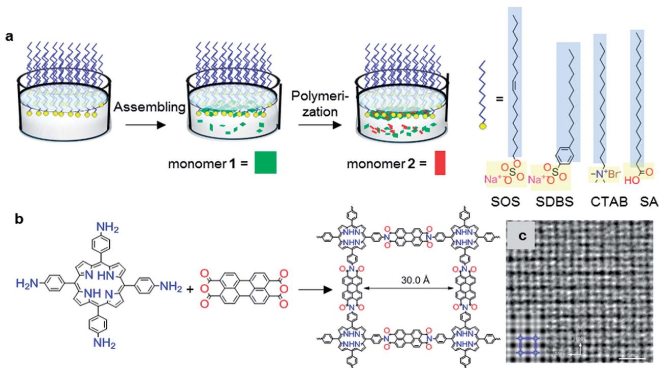
Fig. 3 Synthesis of structurally-ordered 2D polyimide crystal using a novel air-water interface method assisted by surfactant monolayer: (a) synthesis procedures, (b) and reaction scheme with precursors; (c) HRTEM image of resultant 2D polyimide crystals. Scale bar: 5 nm. Adapted from ref. 38 with permission. Copyright © 2019, the author(s), under exclusive licence to Springer Nature Limited.
