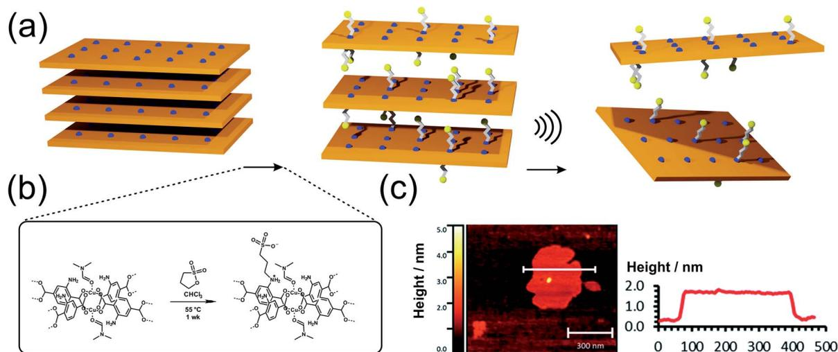
Fig. 5 (a) Schematic depiction of the postsynthetic anchoring of charged sulfonate groups on the backbone of  $\text{Cu}_2(\text{NH}_2\text{-bdc})_2(\text{DMF})_2$  in order to facilitate the exfoliation of the layered structure. (b and c) AFM and height profile of the exfoliated layers. Reproduced from ref. 114 with permission from the Royal Society.
