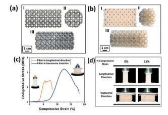
Fig. 2 (a and b) Atomistic model from molecular dynamics simulations and the corresponding ABS 3D printed micro-model one (I: front view; II: top view: III: isometric view). (c) Curves for the uniaxial compressive tests along longitudinal and transverse filter directions. (d) Representative snapshots of the 3D printed model at specific deformation percentages along longitudinal and transverse directions.
