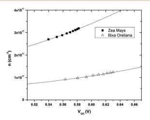
Fig. 9 Electronic density extracted as a function of open circuit voltage with its corresponding adjustment curves according to egn (3).
