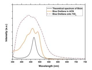
Fig. 4 Experimental absorption spectra of the dye obtained from Bixa orellana in solution and adhered to  $TiO_2$  compared with the theoretical spectrum obtained for bixin.
