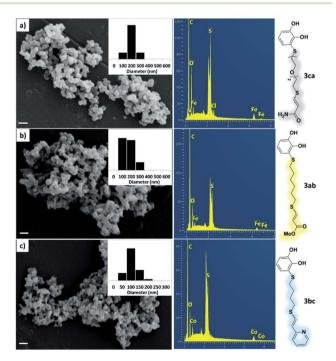
Fig. 2 SEM micrographs, histograms and EDX spectra for CNPs prepared by mixing: (a) **3ca** ligand with Fe(III), (b) **3ab** ligand with Fe(III) and (c) **3bc** ligand with Co(II). Scale bars are 500 nm.
