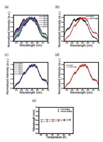
Fig. 2 PL with 532 nm excitation varying temperature. (a) First heating; (b) before and after first heating; (c) second heating; (d) before and after second heating. (e) The emission wavelength of spectra higher intensity for each temperature.
