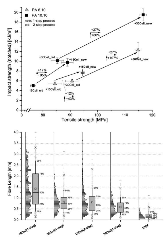
Fig. 7 Influence of the compounding process on the impact strength and tensile strength of PA 6.10 and PA 10.10 composites with 30% cellulose fibres content processed using a twin-screw extruder (top image). Fibre length of PA 6.10 composites with various fibres (cellulose at 15 and 30 wt% vs. 30 wt%) glass fibres (GF) processed by different compounding methods – box plot illustration (bottom image). This figure has been adapted from ref. 99 with permission from Elsevier, copyright 2014.
