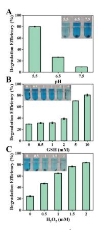
Fig. 5 Degradation of MB using 10 μg mL<sup>-1</sup> biogenic FeS NPs for 4 h treatment. (A) Degradation of MB in buffer solution with various pH values (5.5, 6.5, and 7.5). (B) MB degradation in buffer solution (pH 5.5) with different concentrations of GSH (0, 0.5, 1, 2, 5 and 10 mM). (C) MB in buffer solution (pH 5.5) with different concentrations of H<sub>2</sub>O<sub>2</sub> (0, 0.5, 1, 1.5 and 2 mM).
