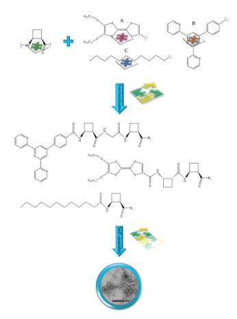
Fig. 4 Examples of cis-ACBC residues functionalized with: (A) TTF, 50 (B) hcptpy,<sup>51</sup> and (C) lipophilic chain<sup>52</sup> self-assembling to form fibrils/fibers.  $R_1 = OMe \text{ and } R_2 = ONa.$
