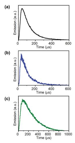
Fig. 4 Kinetic profiles of the emission in channel 2 (C2: 515-580 nm) of (a)  $UC_{Er,2}$ , (b)  $UC_{Ho}$ , and in channel 1 (C1: 420–500 nm) of (c)  $UC_{Tm}$ .  $(\lambda_{\rm exc} = 975 \text{ nm}; F_{\rm d} = 0.2 \text{ J cm}^{-2}).$
