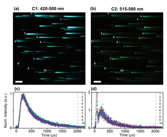
Fig. 6 Equal temporal behavior of several agglomerates of UC<sub>Tm</sub>@Rh110. NIR-LSM images of the same region of UC<sub>Tm</sub>@Rh110 sample under 975 nm excitation ( $F_d = 0.9 \text{ J cm}^{-2}$ ) in (a) channel 1 (C1: 420–500 nm; 560 V) and (b) channel 2 (C2: 515–580 nm; 635 V). Time-resolved normalized intensity profiles of numbered agglomerates in (c) channel 1 and (d) channel 2. Scale bar: 50 μm.
