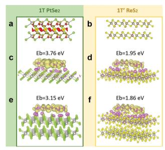
Fig. 1 The interlayer differential charge density of bilayer PtSe2 (a) and bilayer ReS2 (b) calculated by DFT. Side views of the electron density difference isosurface (0.00036 electron bohr<sup>-3</sup>) for MeB molecules absorbed on 1L PtSe<sub>2</sub> (c), 2L PtSe<sub>2</sub> (e), 1L ReS<sub>2</sub> (d), and 2L ReS<sub>2</sub> (f). The binding energy of these systems was calculated respectively.
