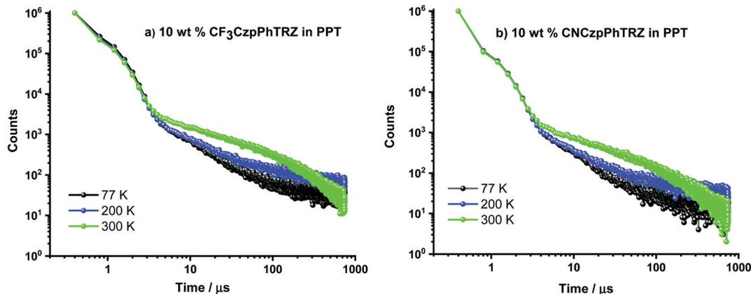
Fig. 5 Temperature-dependent time-resolved photoluminescence lifetime of 10 wt% doped films of (a)  $\text{CF}_3\text{CzpPhTRZ}$  and (b)  $\text{CNCzpPhTRZ}$  in PPT ( $\lambda_{\text{exc}} = 379 \text{ nm}$ ).
