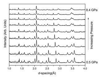
Fig. 3 Neutron diffraction patterns of FePO<sub>4</sub>-II with increasing pressure.
