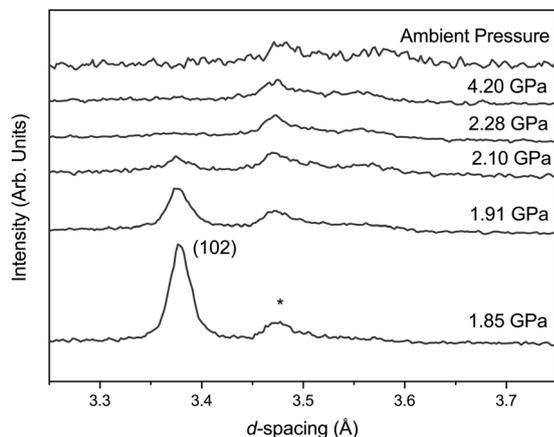
Fig. 2 Neutron diffraction patterns of FePO<sub>4</sub>-I with increasing pressure. The reflection at  $\sim 3.37$  Å is the (102) reflection of FePO<sub>4</sub>-I, the reflection at  $\sim 3.47$  Å is the (asterisk) reflection of the Al<sub>2</sub>O<sub>3</sub> from the anvil and the emerging but broad feature at  $\sim 3.56$  Å can be indexed as the (111) reflection of FePO<sub>4</sub>-II.
