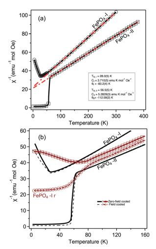
**Fig. 7** Temperature dependence of magnetic susceptibility of FePO $_4$ . (a) ZFC inverse susceptibility of the two phases of FePO $_4$  at ambient pressure, fitted to Curie–Weiss law (red dashed line, see text). (b) ZFC (solid/squares) and FC (dashed/circles) inverse susceptibilities of both phases at ambient pressure, compared with that of the recovered sample (FePO $_4$ -Ir) from 4.2 GPa (red squares and circles) below  $T_{\rm N}$ .
