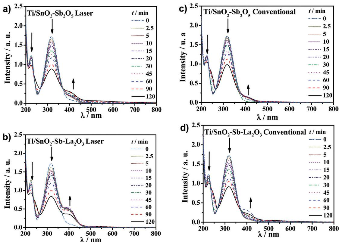
Fig. 9 Evolution of the UV spectra with time during the electrochemical oxidation of 25 mg L<sup>-1</sup> of 4-nitrophenol at 30 mA cm<sup>-2</sup> using the laser-prepared (a and c) and conventionally made anodes (b and d).
