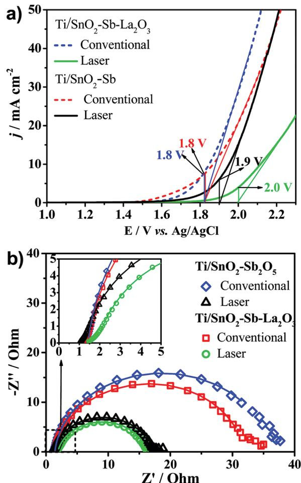
Fig. 6 Linear sweep voltammetry profiles recorded at a scan rate of  $10 \text{ mV s}^{-1}$  (a) and Nyquist plots of the anodes (b) taken at the OER onset potential from 0.1 to  $10^4 \text{ Hz}$  (inset is the expanded view of the high-frequency region). Electrolyte:  $0.5 \text{ mol L}^{-1} \text{ H}_2\text{SO}_4$ .
