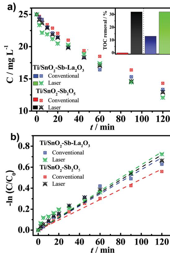
Fig. 8 4-Nitrophenol removal (a) and the kinetics (b) with different SnO<sub>2</sub>-based anodes. Conditions: electrolyte volume: 150 mL,  $j$ : 30 mA cm<sup>-2</sup>, electrolyte: Na<sub>2</sub>SO<sub>4</sub> 0.25 mol L<sup>-1</sup>. Inset: The TOC removal percentages after 120 min of treatment.
