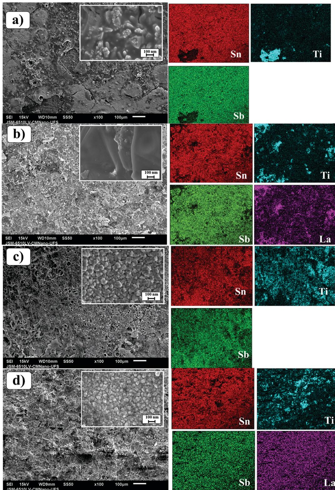
Fig. 2 SEM images of the Ti/SnO<sub>2</sub>-Sb<sub>2</sub>O<sub>5</sub> (a and c) and SnO<sub>2</sub>-Sb-La<sub>2</sub>O<sub>3</sub> (b and d) anodes employing conventional (furnace) (a and b) and CO<sub>2</sub> laser (c and d) heating.
