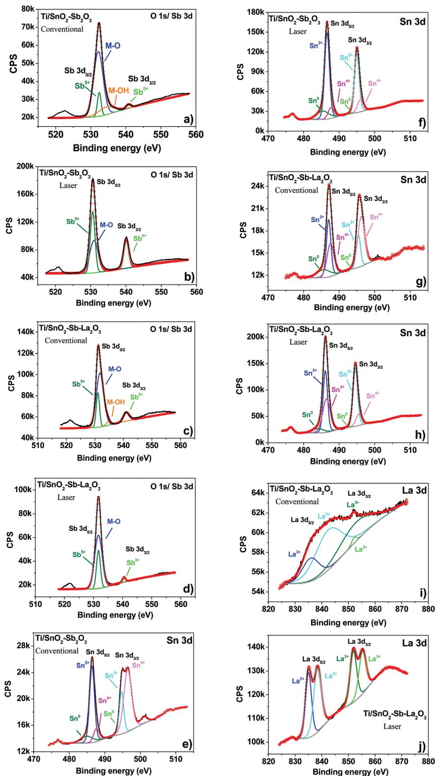
Fig. 4 High-resolution XPS spectrum of O 1s/Sb 3d, Sn 3d and La 3d for Ti/SnO<sub>2</sub>-Sb<sub>2</sub>O<sub>5</sub> electrodes (a and e) conventional, (b and f) laser and Ti/SnO<sub>2</sub>-Sb-La<sub>2</sub>O<sub>3</sub> electrodes. (c, g and i) Conventional and (d, h, and j) laser.
