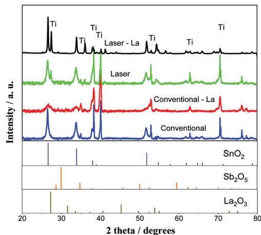
Fig. 1 XRD diffraction patterns of Ti/SnO<sub>2</sub>–Sb<sub>2</sub>O<sub>5</sub> (a) and Ti/SnO<sub>2</sub>–Sb–La<sub>2</sub>O<sub>3</sub> (b) prepared by conventional heating (furnace) and laser heating processes.
