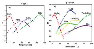
Fig. 3 ZT values of different materials in different temperature ranges (a) for n-type and (b) for p-type materials. Commercial alloys of bismuth and antimony tellurides from Marlow industries (unpublished data); types of doped PbTe;7 skutterudite alloys of CoSb3 and CeFe4Sb12 from JPL, Caltech (unpublished data); TAGS; doped SiGe; Yb14MnSb11; 10 Redrawn from ref. 8
