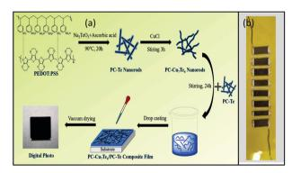
Fig. 14 (a) Schematic of the steps for the fabrication of PC-Cu7Te4/ PC-Te composite film and (b) photograph of a fabricated TE device by using as-prepared film. Reprinted with permission from ref. 159 (Y. Lu, Y. Qiu, Q. Jiang, K. Cai, Y. Du, H. Song, M. Gao, C. Huang, J. He, D. Hu, Appl. Mater. Interfaces. 10 (2018) 42310-42319). Copyright (2018) ACS Publications.
