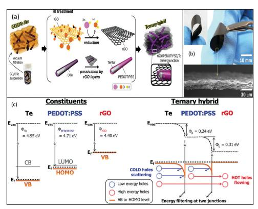
Fig. 13 (a) Synthesis of TE hybrid paper, (b) picture of prepared flexible  $G_{0.1}DTe_{0.9}$  hybrid paper, and (c) energy diagram of the rGO/PEDOT:PSS/TeNW heterojunctions showing energy filtering at two junctions: PEDOT:PSS/TeNW and rGO/PEDOT:PSS of DTe. Reprinted with permission from ref. 157 (J. Choi, J. Y. Lee, S. S. Lee, C. R. Park, H. Kim, Adv. Energy Mater. 6 (2016) 1-8). Copyright (2016) John Wiley & Sons Publications.
