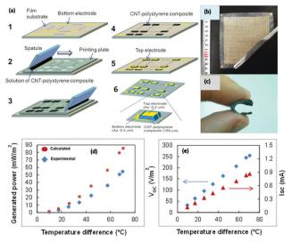
(a) Schematic of the fabrication steps, (b) photograph of a CNTpolystyrene composite film (thickness: 75 μm) fabricated on a film substrate, (c) photograph of the fabricated TEG, (d) graph of the generated power output, and (e) open circuit voltage and short-circuit current with temperature difference. Reproduced from ref. 141 (K. Suemori, S. Hoshino, T. Kamata, Appl. Phys. Lett. 103 (2013)) with the permission of AIP Publishina
