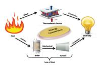
Fig. 1 Schematic representation of electricity generation by comparing the energy conversion between a thermoelectric device and conventional thermal plant.
