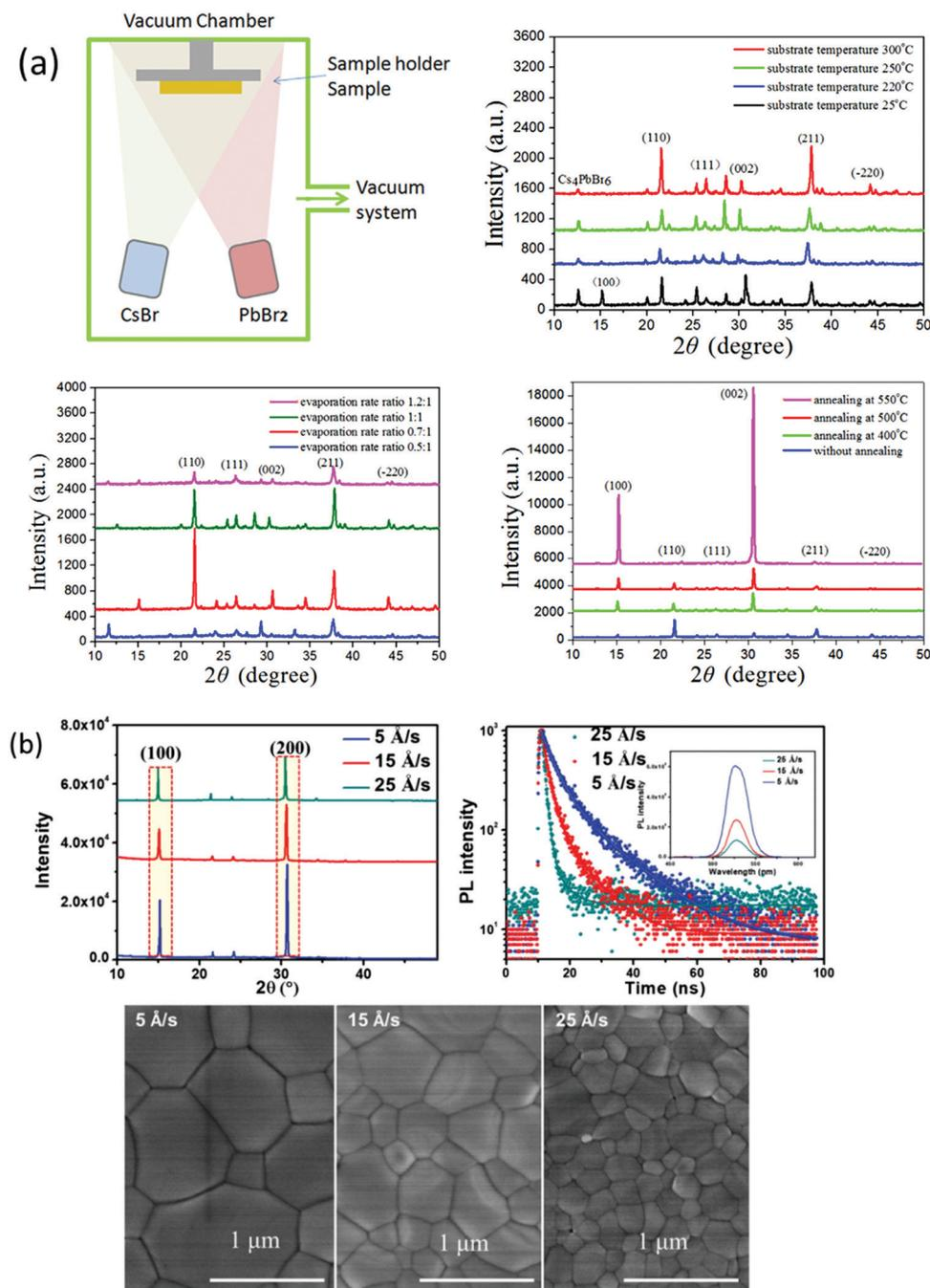
Fig. 10 (a) Representation of the vacuum dual-source thermal co-evaporation process for the preparation of CsPbBr<sub>3</sub> films. Reproduced with permission ref. 124. Copyright 2020, Elsevier Ltd. (b) Corresponding SEM micrographs of the CsPbBr<sub>3</sub> films evaporated at different rates. Reproduced with permission ref. 125. Copyright 2018, Wiley-VCH.
