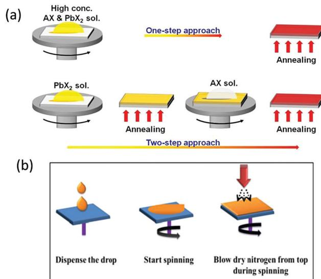
Fig. 6 Representation of one-step and two-step strategies for the preparation of perovskite films. AX and PbX<sub>2</sub> symbolize CsBr and PbBr<sub>2</sub>, respectively. Reprinted with permission ref. 106. Copyright 2019, The Royal Society of Chemistry. (b) N<sub>2</sub> gas flow-assisted method for the fabrication of pinhole-free CsPbBr<sub>3</sub> thin films. Reprinted from ref. 119. Copyright 2020, Gupta, Kulbak, and Cahen.
