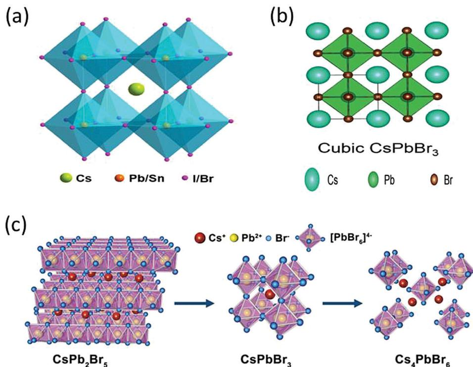
Fig. 2 (a) The crystal structure of an inorganic CsPbX<sub>3</sub> (X = I, Br, Cl) perovskite. Reprinted with permission ref. 83. (b) Cubic structure of CsPbBr<sub>3</sub>. Reprinted with permission ref. 84. Copyright 2019, The Royal Society of Chemistry. (c) Three-dimensional crystal structure models of CsPb<sub>2</sub>Br<sub>5</sub>, CsPbBr<sub>3</sub>, and Cs<sub>4</sub>PbBr<sub>6</sub> structures. Reprinted with permission ref. 120. Copyright 2019, American Chemical Society.
