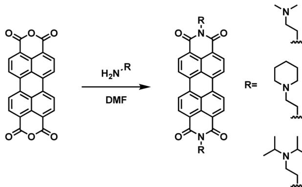
Scheme 1 Reaction scheme for the synthesis of self-doped PDIs.
