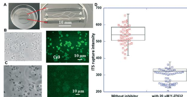
**Fig. 8** (A) Picture of one blood-vessel-mimicking chip and its close-up photo; (B) optical micrograph and fluorescence image of the integrin tension sensors without inhibitor (Y-27632) treatment; (C) optical micrograph and fluorescence image of the integrin tension sensors with  $20 \mu\text{M}$  inhibitor (Y-27632) treatment. (D) The measured fluorescence intensity with and without inhibitor (Y-27632) treatment.
