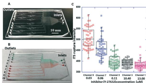
**Fig. 9** (A) Photo of one microchip with 10 blood-vessel-mimicking channels with a solution concentration gradient generator; (B) optical micrograph showing different concentrations of the inhibitor (food dyes were used for visibility) flowed into 10 blood vessel mimicking channels (channel # 1–10); (C) the measured fluorescence intensity with inhibitor (Y-27632) treatment of different concentrations automatically generated by the solution concentration gradient generator on chip.
