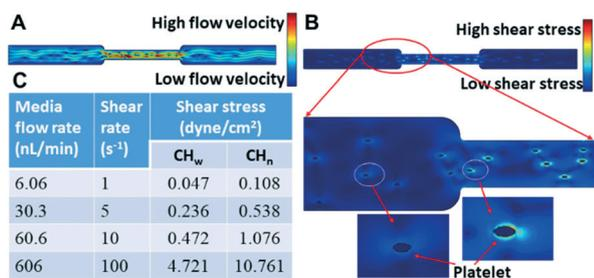
**Fig. 4** (A) Representative velocity profile inside the wide and narrow microchannels. (B) Representative flowing shear stress profile inside the wide and narrow microchannels. (C) The calculated flowing shear stress on the platelets at different solution flow rates into the chip and the different regions of the microchannels.
