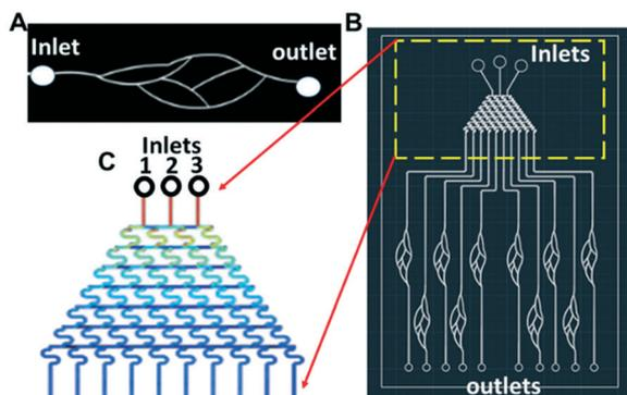
**Fig. 3** (A) Sketch of a single blood vessel mimicking chip. (B) Sketch of a chip consisting of ten blood vessels integrated with a solution concentration gradient concentration generator. (C) Close-up of the solution concentration gradient generator with three inlets.
