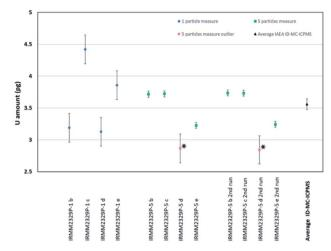
Fig. 9 Total U mass per particle and combined uncertainty (k = 1) in IRMM-2329P reference material as measured at IAEA-SGAS using ID-MC-ICPMS. \*Note that the IRMM-2329P-5-d 1st and 2nd run samples were considered as containing only 1 particle instead of 5, and thus not taken into account into final average of the uranium amount.
