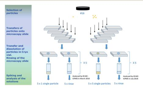
Fig. 6 Flowchart of the sample preparation for the verification measurements of the IRMM-2329P at IAEA-SGAS. The particle transfers were performed by JRC-Geel G.2.
