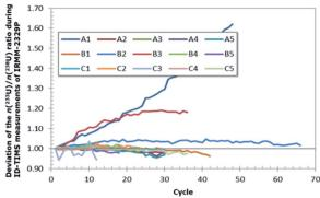
Fig. 5 TIMS measurements of the  $n(^{233}U)/n(^{238}U)$  ratio of filaments of the first IRMM-2329P turret, showing the drift of the measured  $n(^{233}U)/$  $n(^{238}\text{U})$  ratio from the initial  $n(^{233}\text{U})/n(^{238}\text{U})$  measured at the beginning of the measurement cycle. It can be seen on the graph that only two filaments (A1 and B3) showed a drift exceeding 10% of the initial value, and were therefore discarded as outliers
