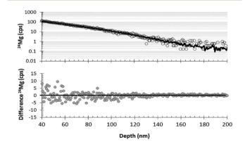
Fig. 7 Graphs demonstrating the quality of SRIM-fit to a measured DLC profile (SW\_3) for the last 160 nm of the <sup>24</sup>Mg depth profile. Top: raw data (circles) plotted with SRIM best–fit curve (line); bottom: the difference between SRIM and the raw SIMS data.
