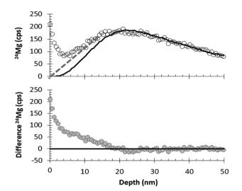
Fig. 8 Illustration of DLC surface correction using measured data (circles, SW\_3) vs. SRIM best fit (solid line) for the first 50 nm of the  $^{24}$ Mg depth profile. Top: comparison of raw data with the SRIM best-fit curve; dashed line gives an example of a (previously used10) visual correction based only on curve shape. Bottom: the difference between SRIM and the raw SIMS data.
