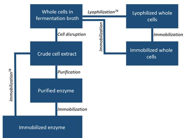
**Fig. 5** Possible enzyme formulations and how they can be prepared from cultivated cells. Whole cells can be used directly as the catalyst, or be lyophilized or immobilized. Otherwise, cells can be disrupted to obtain cell free extract, which can be purified or (directly) immobilized.
