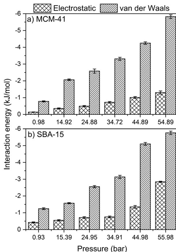
Fig. 10 The electrostatic and van der Waals interaction energy associated with the adsorption of CO<sub>2</sub> molecules on the surfaces of MCM-41 and SBA-15 materials as a function of pressure are shown. These analyses are performed on data averaged over the last 10 ns of the simulation time. The error bars are calculated based on the simulations performed in triplicates.
