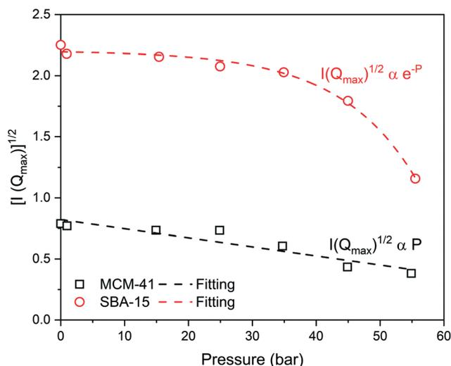
Fig. 4 The amplitudes of the SANS intensity  $[I(Q_{\text{max}})]^{1/2}$  at the maximum of the first-order peak as a function of the applied pressure in MCM-41 and SBA-15 pores are shown. The pressures at which the intensity reaches zero average contrast in MCM-41 and SBA-15 are about 110 bar and 72 bar, respectively.
