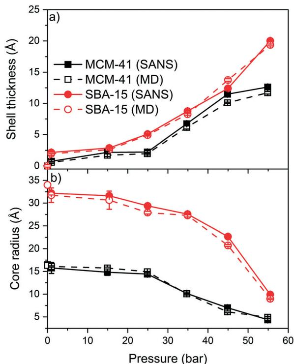
Fig. 7 The thickness of the adsorbed  $\text{CO}_2$  layer determined from the small-angle neutron scattering measurements and molecular dynamics simulations (a) and the corresponding core radius (b) as a function of the applied pressure are shown. The error bars of the SANS and MD data represent standard deviations based on fittings and simulations performed in triplicates.
