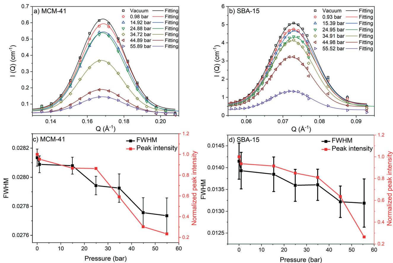
**Fig. 3** The fitted first-order peak intensity of MCM-41 and SBA-15 as a function of the applied pressure are represented in (a) and (b), respectively. The full width half maximum (FWHM) and the peak intensity normalized by the intensity of the pore under vacuum for MCM-41 and SBA-15 are shown in (c) and (d), respectively.
