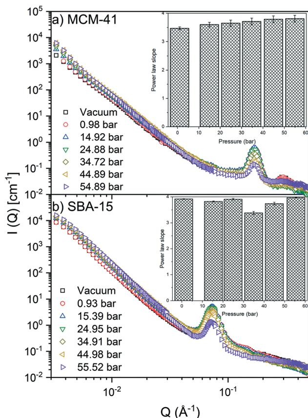
**Fig. 2** The small-angle neutron scattering intensities of  $\text{CO}_2$ -loaded (a) MCM-41 and (b) SBA-15 pores as a function of the wavevector and the applied pressure are shown. The insets represent the power law slope values as a function of the applied pressure.
