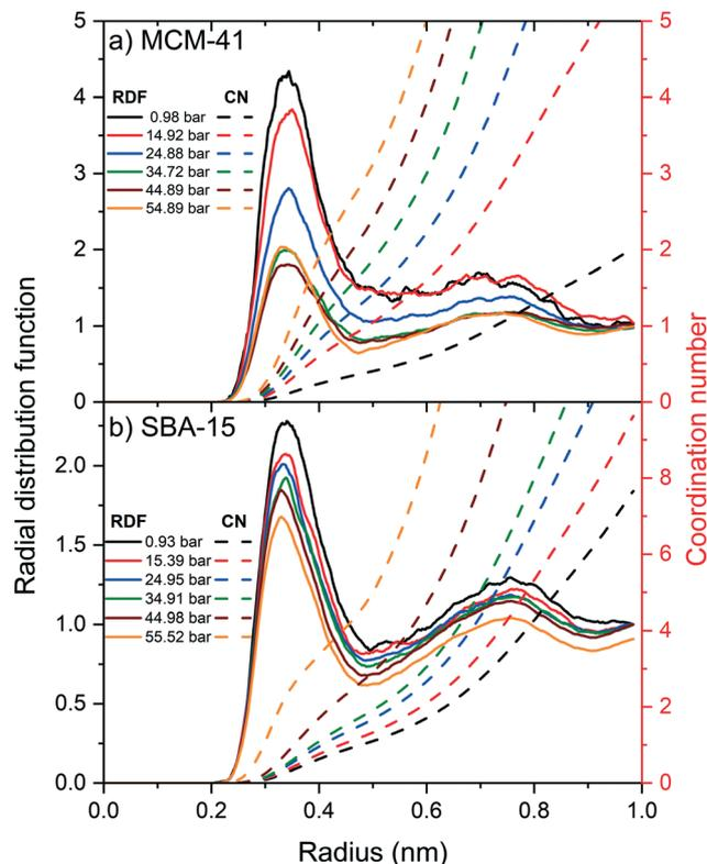
Fig. 8 The radial distribution functions and the corresponding coordination numbers of  $-\text{OH}-\text{CO}_2$  in the MCM-41 (a) and SBA-15 (b) as a function of the applied pressure are shown. The simulation data are averaged over the last 10 ns of the simulation time.
