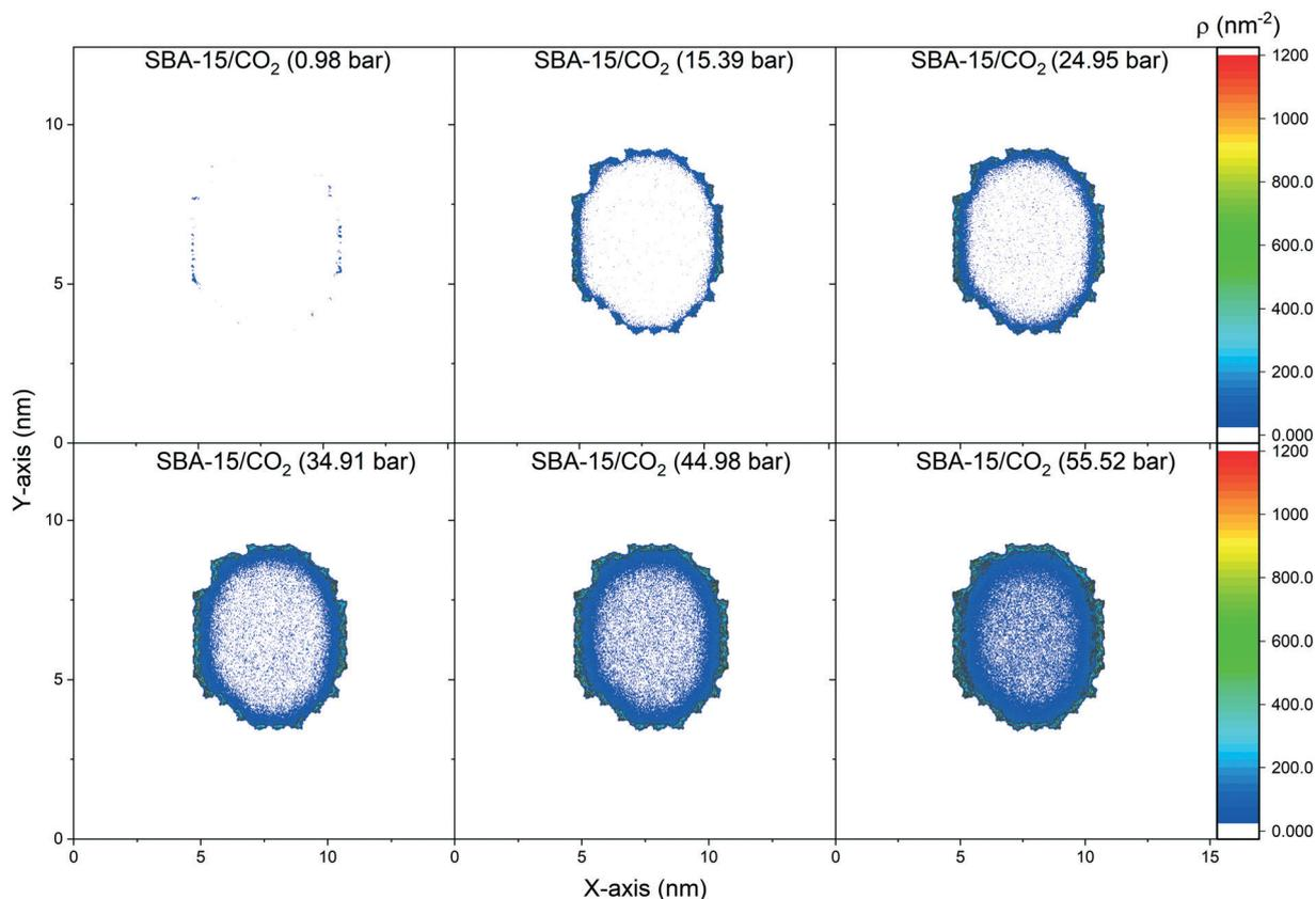
**Fig. 6** The 2D density maps of the CO<sub>2</sub> molecules adsorbed on the pore walls of SBA-15 as a function of the pressure obtained from the classical molecular dynamics simulations are shown. The pore diameter of SBA-15 is 6.8 nm. The density maps are averaged over the last 10 ns of the simulation time.
