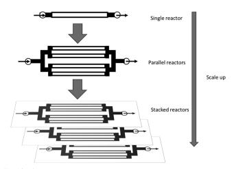
Fig. 10 Scaling up and scaling out of  $\mu$ -IMERs
