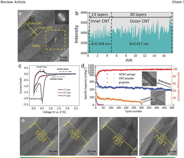
Fig. 20 (a) TEM image of a CNT. (b) Line profile obtained from the wall of a CNT. (c) CV curves of CNT sponge at 0.3 mV s<sup>-1</sup>. (d) Cycling performance of CNT sponge, commercial CNT powder and graphite electrodes at a current density of 100 mA g<sup>-1</sup>. (e) Ex situ TEM images of the CNT structure at different potassiation and de-potassiation potential in the first cycle. Reproduced from ref. 344 with permission from Wiley-VCH.
