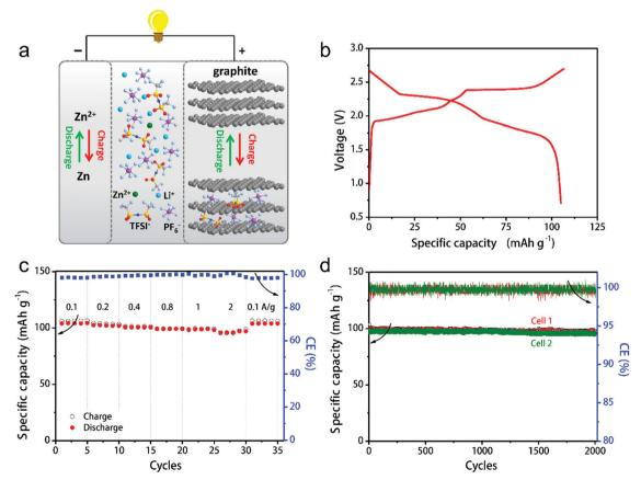
Fig. 31 (a) Schematic illustration of the Zn-graphite battery configuration and electrode reactions. (b) Typical charge-discharge curve at 100 mA  $g^{-1}$ , (c) rate capability and (d) cycling performance of the Zn-graphite battery at 1000 mA  $g^{-1}$ . Reproduced from ref. 431 with permission from Wiley-VCH.
