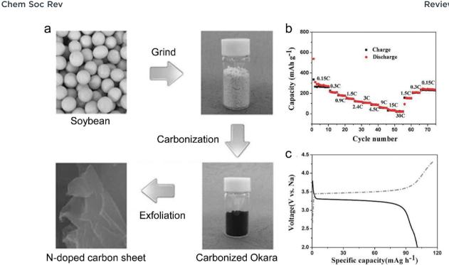
Fig. 17 (a) Schematic representation of the preparation of N-doped carbon sheets. (b) The capacity retention of the N-doped carbon sheets at current densities from 56.25 mA  $\rm g^{-1}$  to 11.25 A  $\rm g^{-1}$ . (c) Charge and discharge curves of the carbon sheets//Na<sub>3</sub>V<sub>2</sub>(PO<sub>4</sub>)<sub>3</sub> sodium ion batteries at 562 mA  $\rm g^{-1}$ . Reproduced from ref. 316 with permission from Wiley-VCH.
