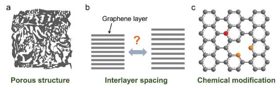
Fig. 3 Common strategies to modify carbon materials, including (a) pore construction, (b) interlayer spacing engineering, and (c) chemical modification.
