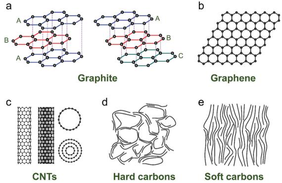
Fig. 2 Typical structures of (a) graphite, (b) graphene, (c) carbon nanotubes, (d) hard carbon, and (e) soft carbon.
