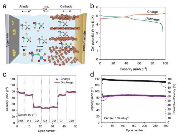
Fig. 28 (a) Schematic of the charging process in a K//C DIB. Fluorine, oxygen, sulfur, and nitrogen atoms in the FSI<sup>-</sup> anion are shown in brown, red, blue, and green colors, respectively. (b) Typical galvanostatic voltage profile of a K//C DIB measured at a current density of 50 mA  $\rm g^{-1}$ . (c) Rate capability measurements and (d) cycling performance of a K//C DIB. Reproduced from ref. 167 with permission from Springer Nature
