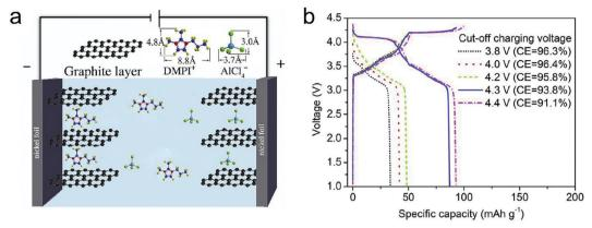
Fig. 32 (a) Operation principle of the DIB containing (DMPI<sup>+</sup>)(AlCl<sub>4</sub><sup>-</sup>) as an IL electrolyte. (b) Charge/discharge curves of the DIB cell at cut-off charging voltages of 3.8-4.4 V. Reproduced from ref. 439 with permission from Elsevier.
